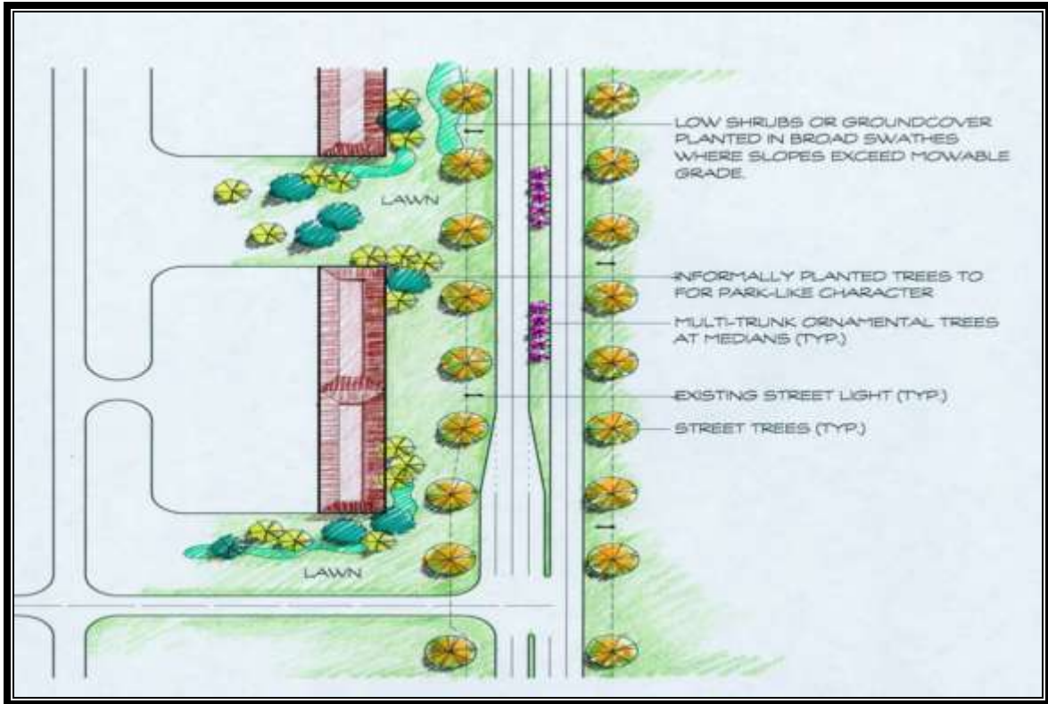
Exhibit ES-5 – Typical Landscaping Near Commercial Development
